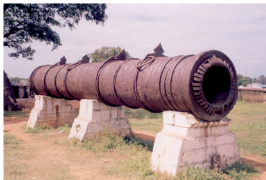
Metallurgy of Ancient Indian Iron and Steel. Fig. 8 The massive forge-welded iron cannon called Rajagopala located at Thanjavur.
